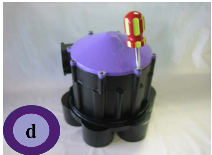
Replace valve top
